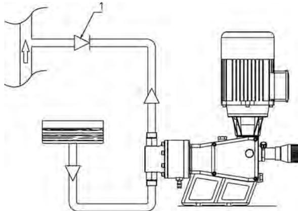
Fig. 13 – Injection valve installed in the discharge hose
