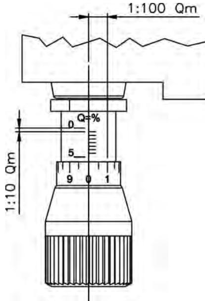
Fig. 16 – Micrometer adjustment
