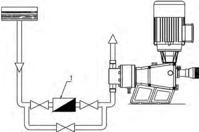
Fig. 12 – Layout for dosing liquids with impurities
