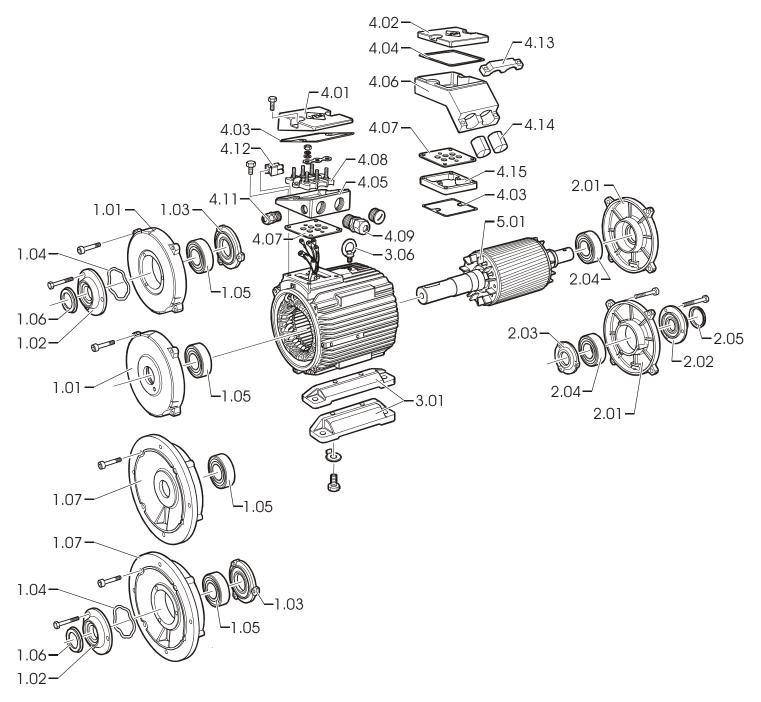
Three-phase motors of the series Y..O have, except the terminal box location at the N-end, the same design
